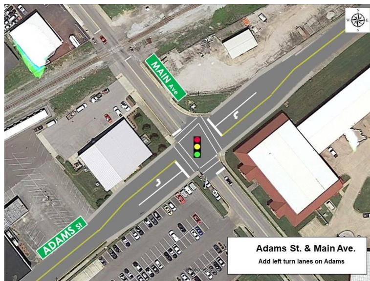
Figure ES-4: Improvement Concept 2: Two-way with left-turn lanes at traffic signals on Adams Street
